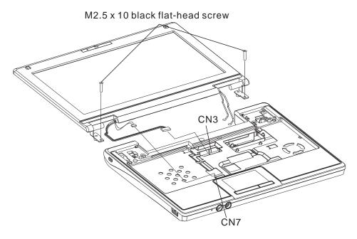
Figure 4-9 Removing the display assembly.
